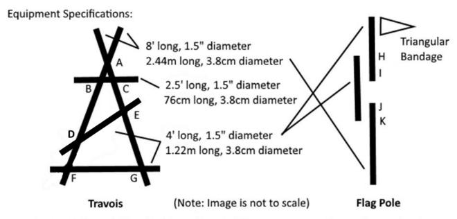
Letters A through K are lashing points. A different rope must be used at each point.
